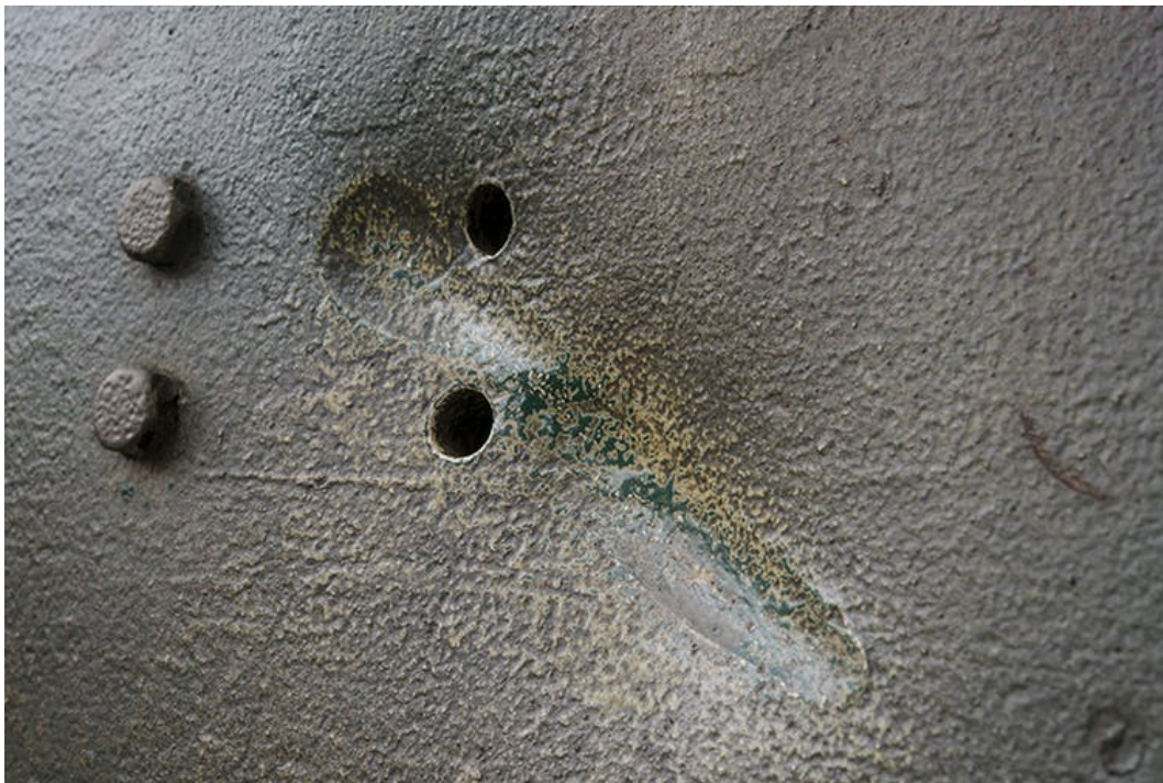
Large calibre impact strikes on Mephisto, possibly made by a French 35mm gun. Queensland
